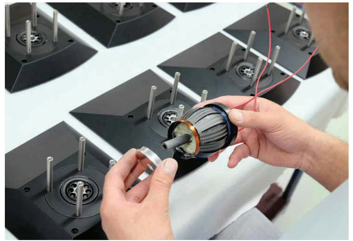
MBL midrange spider-free voice coil and carbon-made centre rod prepared for magnet assembly
