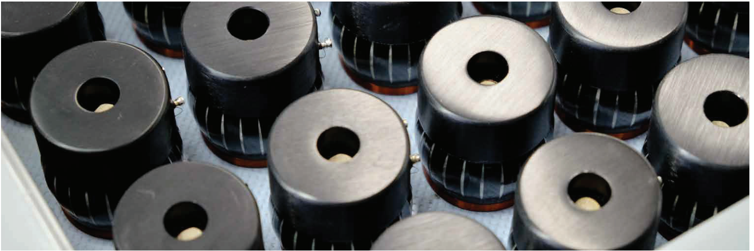
MBL tweeters with aluminium cover plate about to be measured for perfect matching
