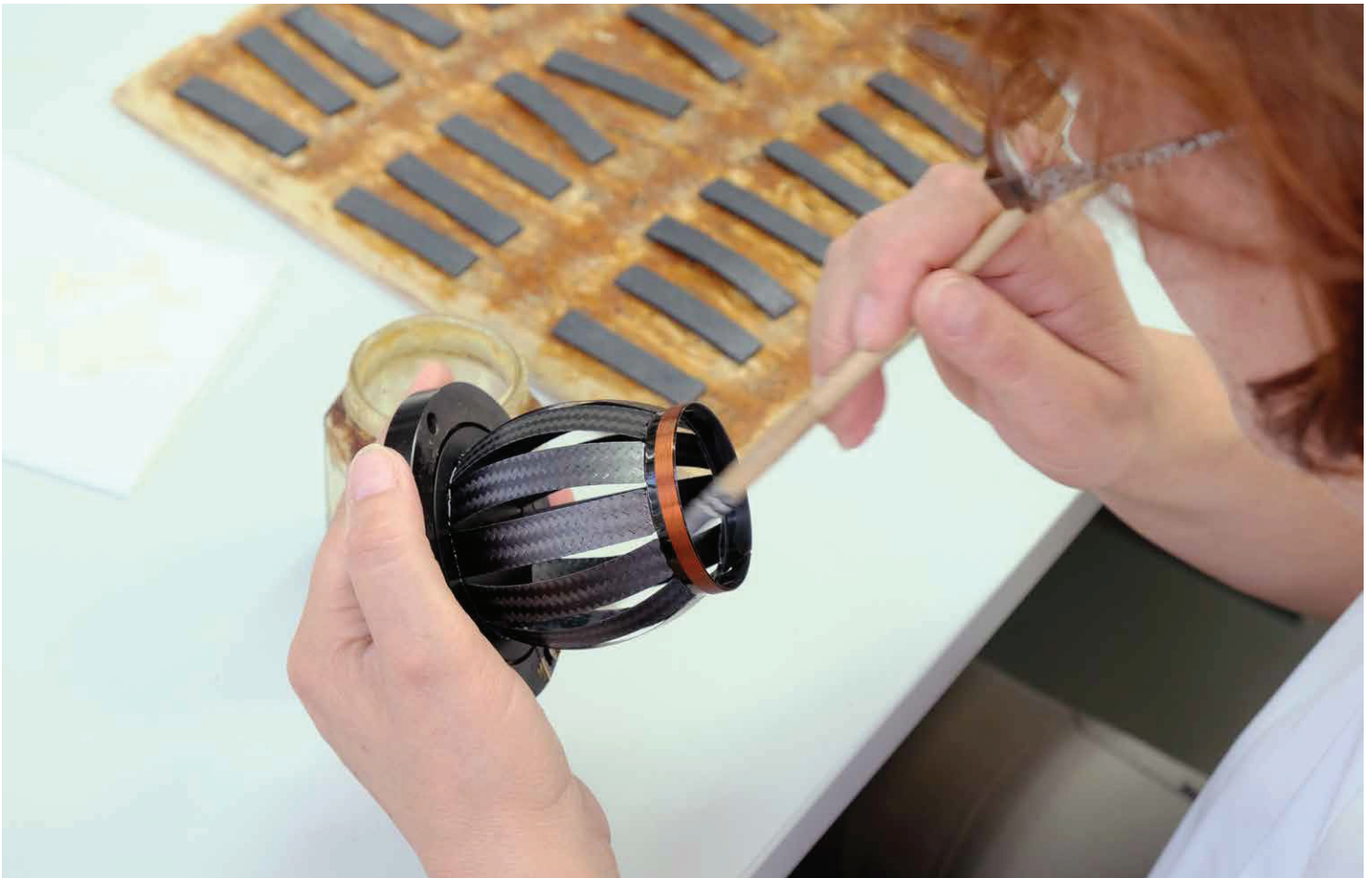
Silicone and sound dampening foam added to the inside of midrange's woven carbon fiber segments
